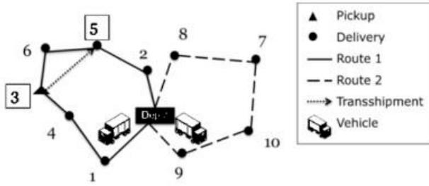
Fig. 1 An illustration of the vehicle routing with transshipment (VRPT)
