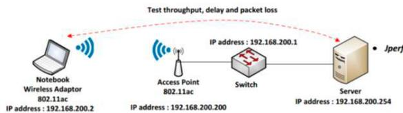
Fig. 2 IPv4 Performance Test
