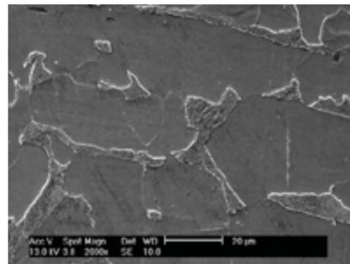
Fig. 5 SEM micrograph of the mold, showing grain in the S400 substrate area
