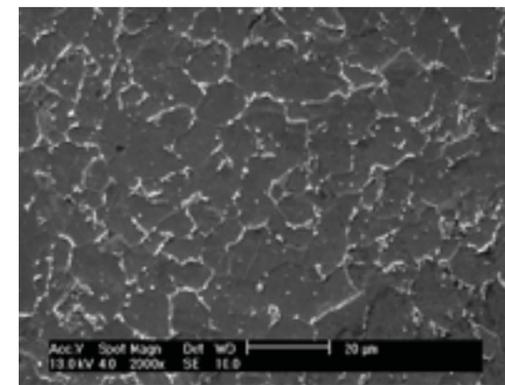
Fig. 7 SEM micrograph of the mold, showing grain in the electrode area
