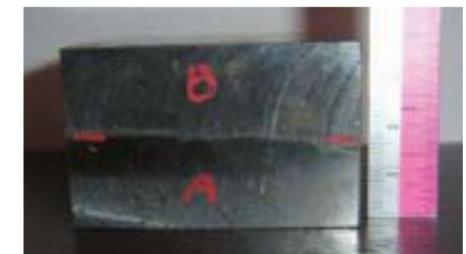
Fig. 2 Cross section of core part of the mold, showing substrate and deposited electrode, designated as region A and B, respectively
