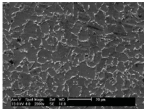
Fig. 6 SEM micrograph of the mold, showing grain in the interface area
