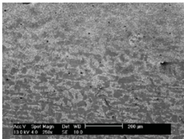
Fig. 4 SEM micrograph of the mold showing small pores in the sample
