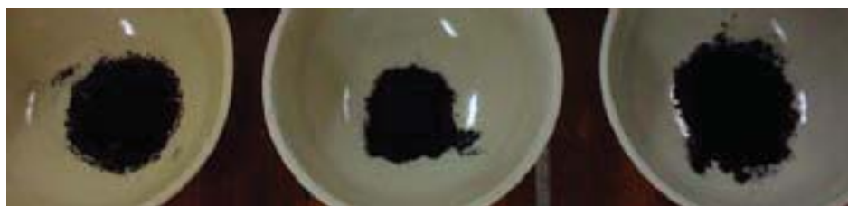
Fig. 2 Powder prepared with f/o = 1:3, 1:1 and 3:1 (from left to right) upon heating at 900°C
