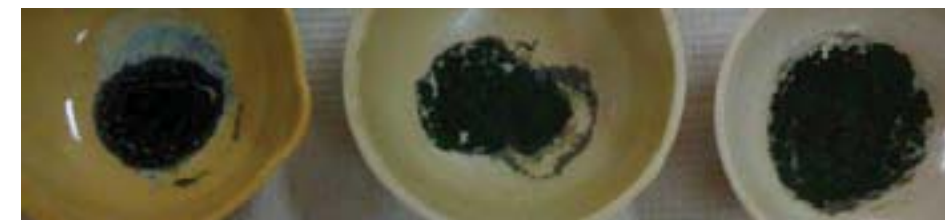
Fig. 3 Powder prepared with f/o = 1:3, 1:1 and 3:1 (from left to right) upon heating at 950°C
